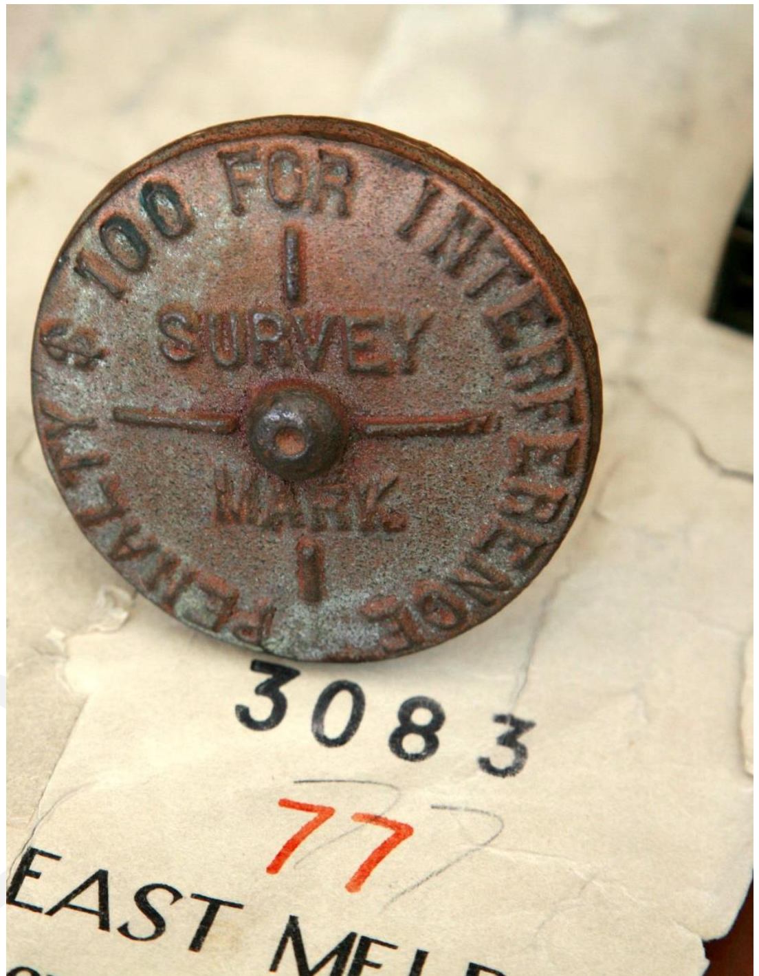
Figure 6: Example of a survey mark – Survey marks out in the field are often not easily distinguishable to the untrained eye.
